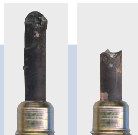
Poor engine performance due to melted or broken heating element
