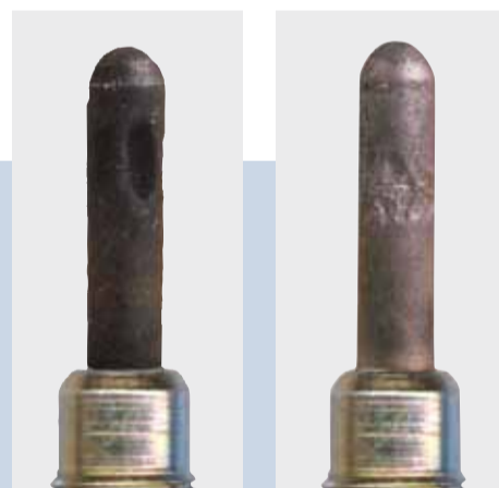
Dents and creases on the heating element causing starting problems
