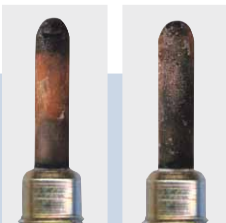
Starting problems due to an overheated or corroded heating element tip
