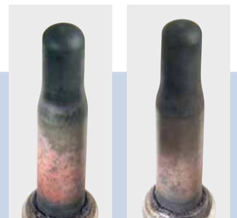
If the glow plug has no continuity, the engine will start poorly or not at all
